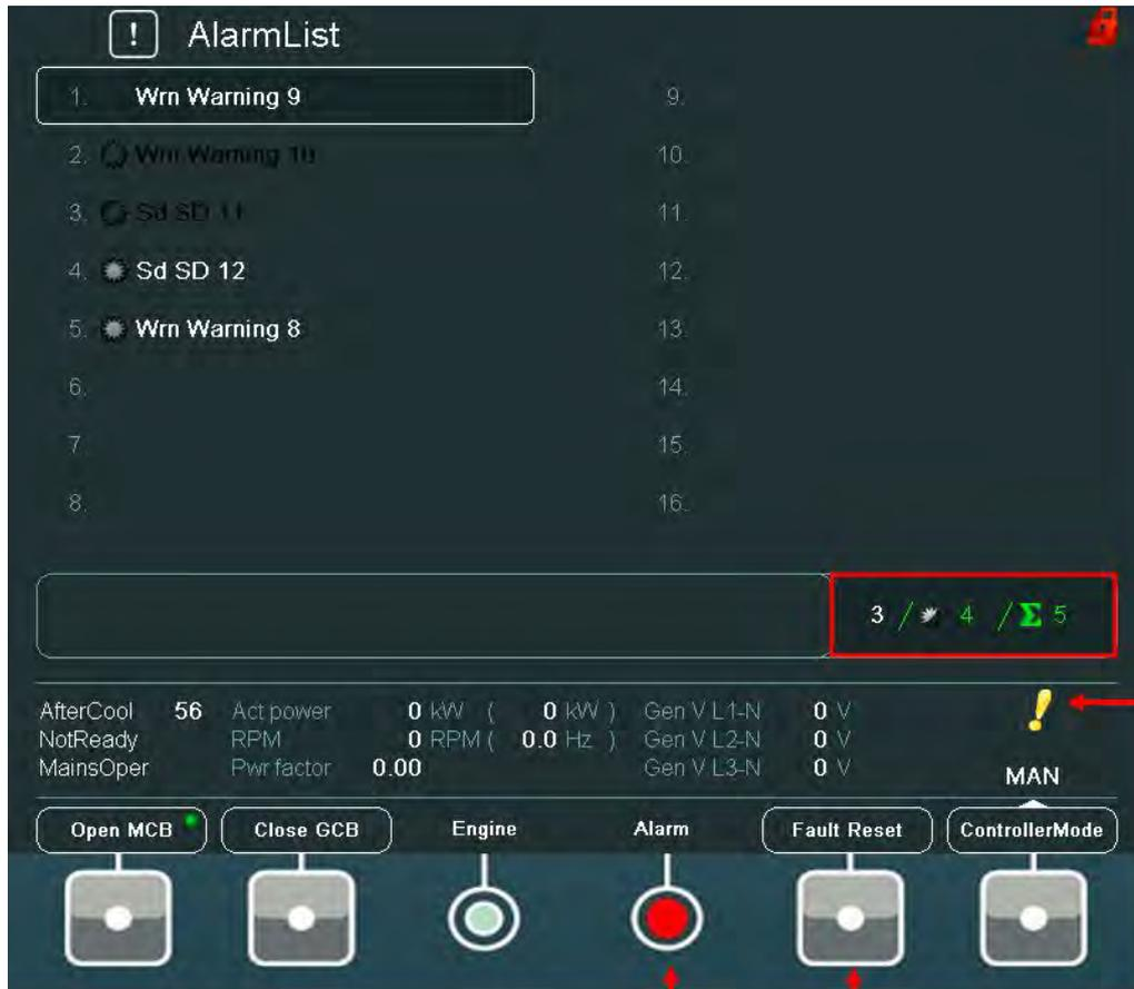
2. Press **Fault Reset** button to confirm all alarms. The **Alarm** LED will stop blinking.
